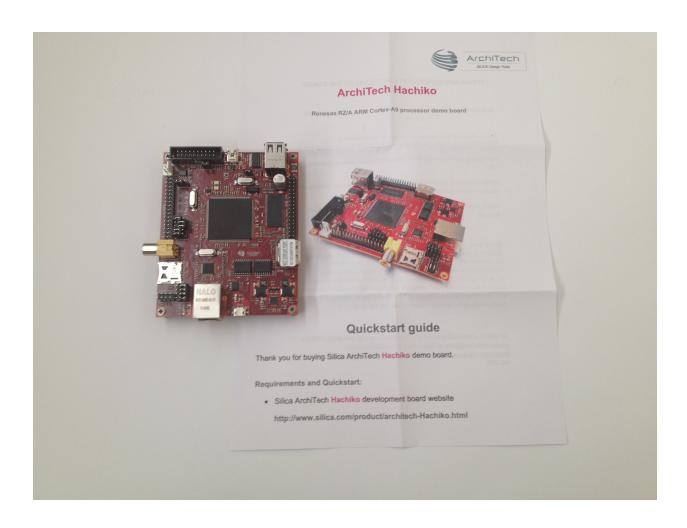
The board itself has been programmed to boot to a Linux console of a really tiny distribution, custom tailored to fit the 10MB of internal ram of Renesas's SoC.
